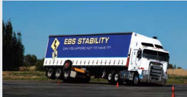
TEST: J turns @ 55KPH with ESP
